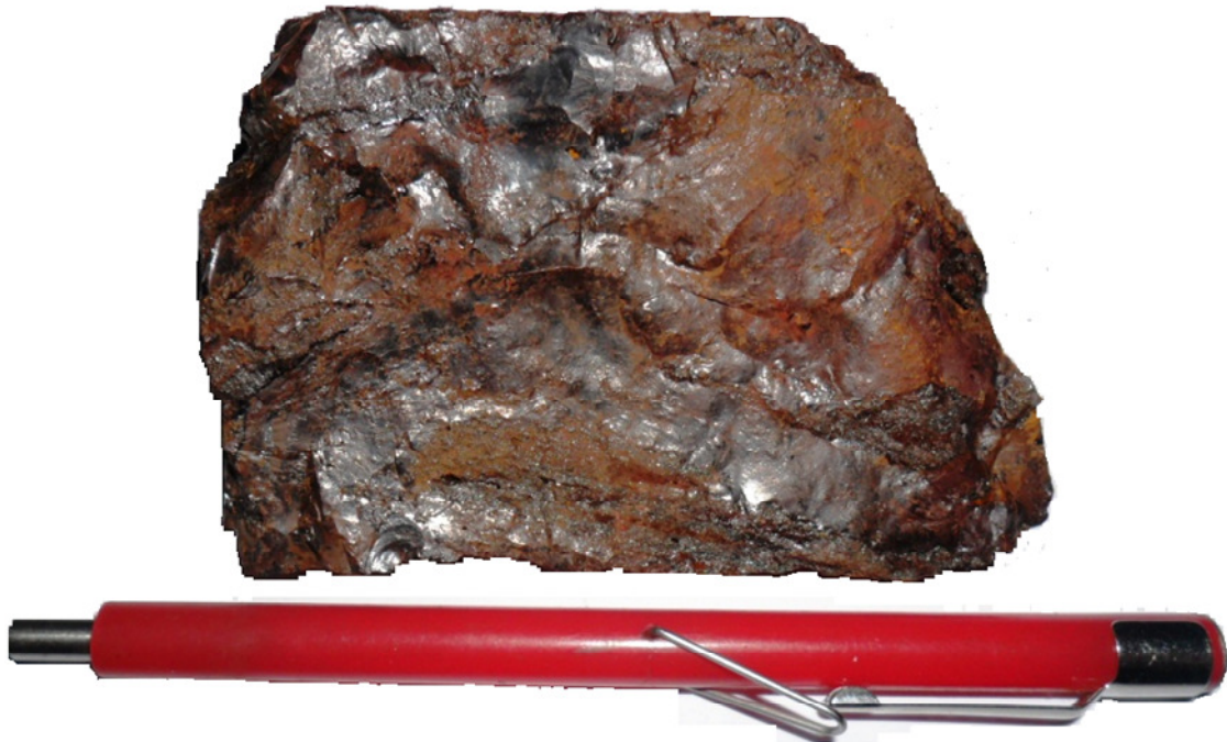
Figure 7.9 Grab sample G01. It was initially thought to be re-crystallised hematite because of its glassy texture but found to contain significant amounts of goethite.
