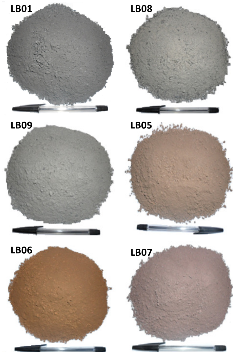
Figure 6.3 Crushed core samples for LB01, LB05, LB06, LB07, LB08 and LB09. LB08 and LB09 are magnetite poor BIF samples whereas LB01 is a magnetite rich sample. Note the difference in colour between the magnetite rich and poor samples. The magnetite hematite sample (LB05), hematite magnetite sample (LB06) and hematite sample (LB07) show colour variations which are due mainly to the alteration of magnetite through to goethite and then to hematite.
