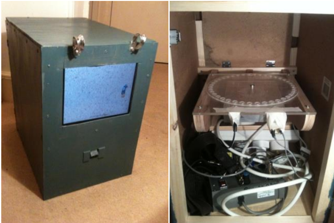
Fig. 1: The DogBox. The front view (left picture) shows the iPad™ in situ displaying a moving stimulus, the reward chute at bottom centre, and the hooks at the top used to attach it to the front of an animal enclosure such as a dog kennel. The inside view (right picture) shows the electronic reward dispenser with space for 40 small liver flavoured dog treats (Barker and Barker little liver treats™). Total of 60 rewards used in experiment 4, with dispenser refilled part-way through each session.
