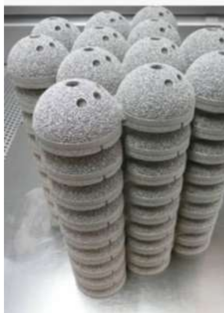
Figure 2.9. Accetabular cups produced in titanium alloy using Electron Beam Melting [25]
