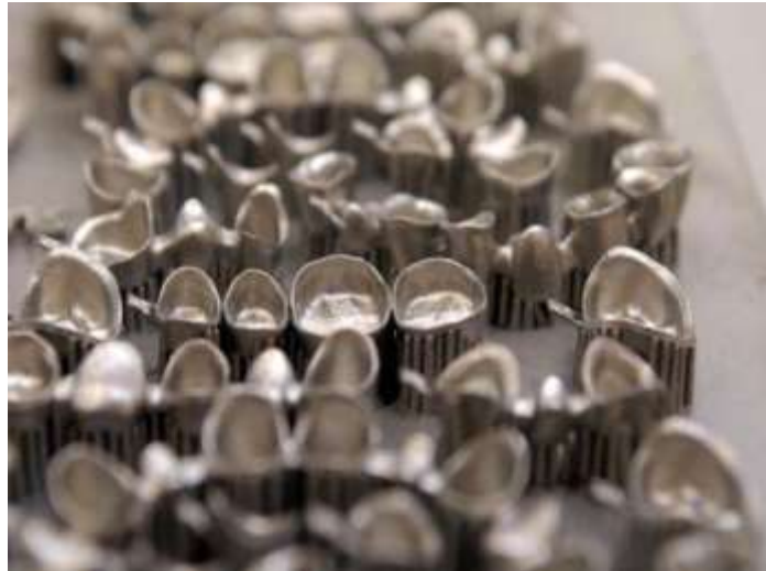
Figure 6.1 Dental copings produced at Renishaw on DMLS M270 (courtesy of Renishaw)
