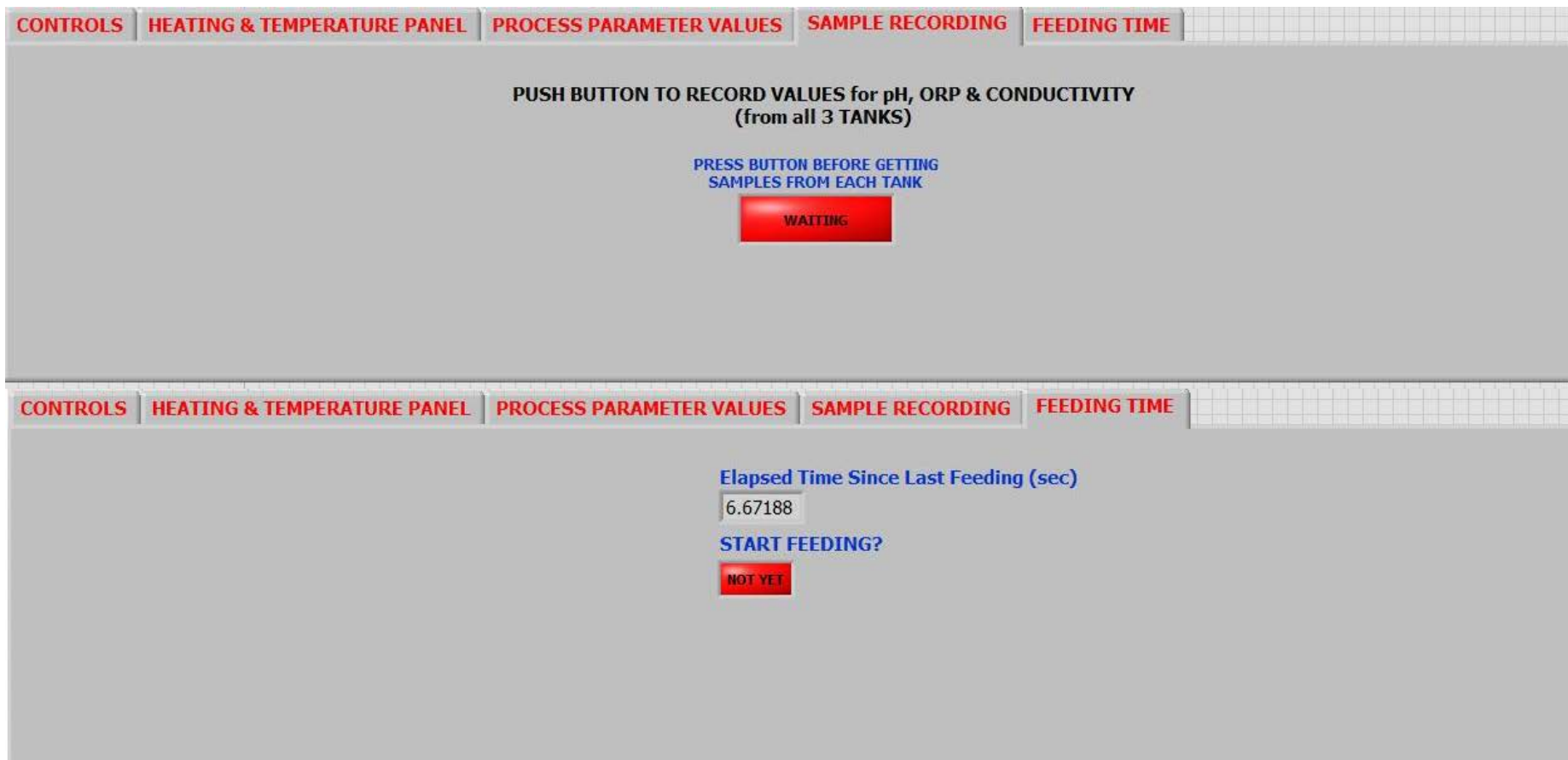
Figure A.6 'Sample recording' tab contains a button to record continuous process parameter data while sampling and 'Feeding time' tab displays the elapsed time since last feeding. The 'Start feeding?' button enables the user to override the feeding regime that is configured at the background.
