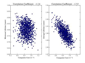
Figure 2: Correlation between objectives and composite cost. Scatter plots show (right) the composite cost and true average lifetime  $f_1(R)$  and (left) minimum lifetime  $f_2(R)$  for 1000 randomly generated routing schemes with random residual charges at the nodes.
