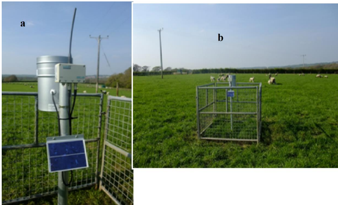
Figure 3.14 a-b: Adcon RG1 double tipping bucket system rain gauge; (b) shows the protective metallic housing from animals' attacks .
