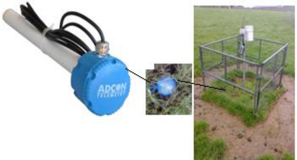
Figure 3.17. Adcon SM1 soil temperature and moisture sensor (calibrated to measure soil temperature at 15cm and soil moisture at 10, 20 and 30 cm in the study area).
