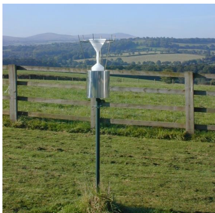
Figure 3.15. The UK Environmental Change Network's bulk precipitation collector in Field 4 (Burrows) of the North Wyke Farm Platform.
