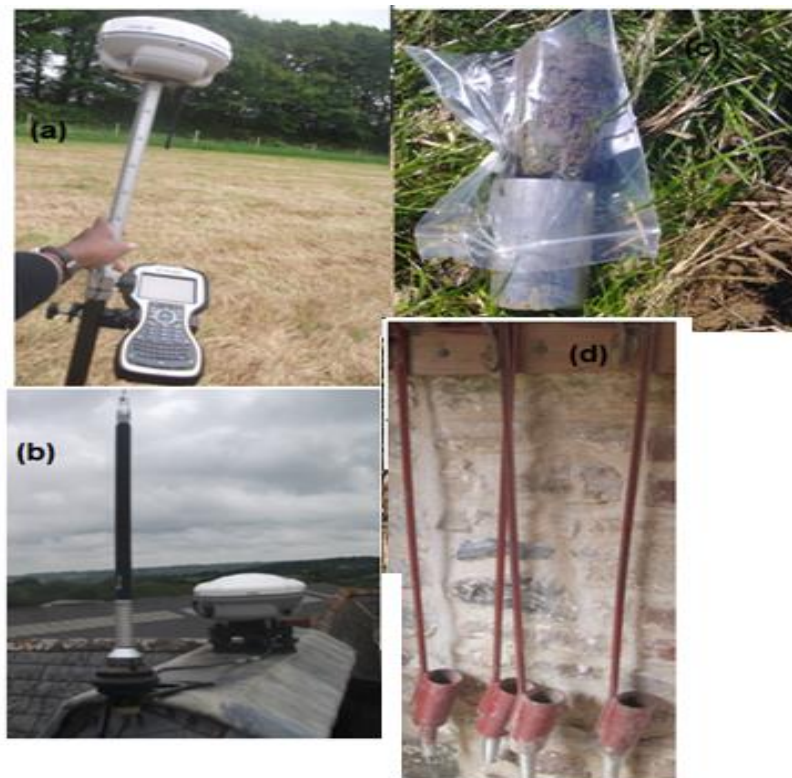
Figure 3.19 a-d. Equipment used for soil sampling. a) Antennae with the detachable receiver Trimble GPS for siting where sample should be taken, b) the GPS base station which is radio-linked with the receiver for the real time kinematic site location (survey). c) A 5.5 by 10 cm cylindrical core and sample for bulk density determination, and d) 2 by 10 cm grass plot samplers.
