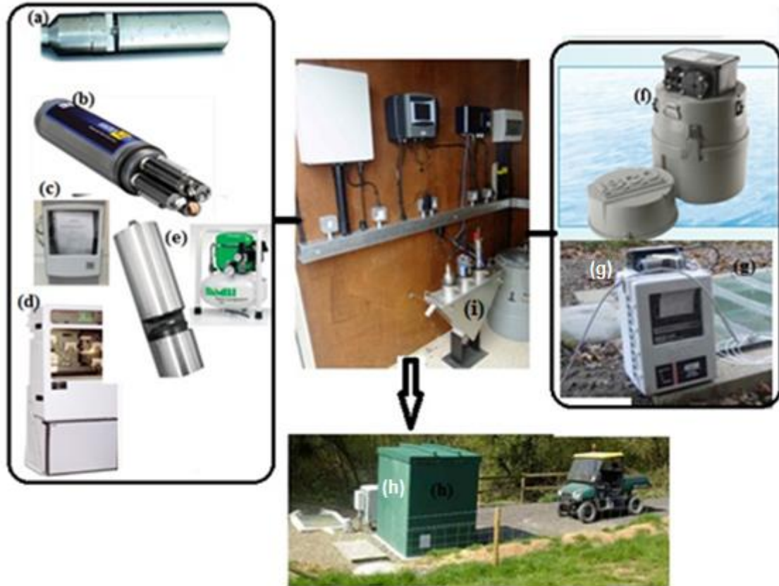
Figure 3.13 a-g: Sensors for monitoring the runoff chemistry and flow in each field of the North Wyke Farm Platform: (a) . is the Nitratax plus sc' for nitrate determination, (b) . is the Multi-parameter water quality sonde for determination of temperature, pH, turbidity, dissolved oxygen and conductivity; it is fixed in the flow cell (i) , (c) and (d) are Phosphax Phosphate analysers for Ortho-P and Total-P, respectively. Phosphate analyser is installed in FP2, FP5 and FP8 only but their data were not used in this study; (e) is ProPS-UV process photometer for determination of dissolved organic carbon; (f) is a sequential or composite sampler for event-based grab samples; (g) is the Bubbler flow meter for discharge measurement; and (h) is the chamber that houses the monitoring equipment.
