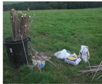
(j). The usual field companions; pegs, sampling cores, plot samplers, spade and soil samples.
