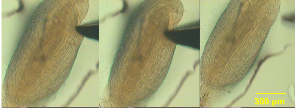
Figure 5.7. PC extracted from the heel area of the hind foot of a 5-year-old Shire horse . Indentor diameter 604 \mu\text{m} . Mechanical deformation of the lamella structure produced by microindentation; the right panel shows restoration of shape when the probe is removed, presumably due to lamellae stiffness and the resilience of the collagen fibril network. Apart from the recoil the main point of interest is that the lamellae only \sim 1 indentor diameter away from the site are completely unaffected by a rather large indentation of almost 1/3 diameter of the corpuscle
