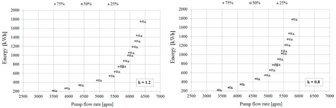
Fig. 3 Energy consumption related to pump station flow rate for all the pump combinations and two demand patterns, obtained fixing three different initial tank water levels (75%, 50% and 25% of the maximum tank water level).
