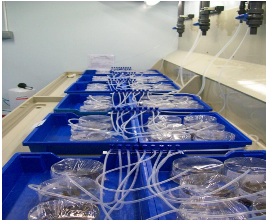
Figure 5.2 The juveniles G. pulex divided into two groups in hard water (150 ppm as \text{CaCO}_3 ) and another group in soft water (15 ppm as \text{CaCO}_3 ), 9 replicates, ( n = 5 per dish), in Aquatic Resource centre laboratories.
