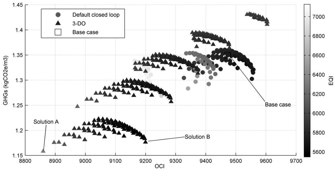
**Figure 4** WWTP performance with adjusted reactor 5 DO setpoint in the 3-DO control strategy and adjusted wastage flow rates in both (compliant solutions only); colour denotes EQI, with a darker shade representing a better quality effluent.
