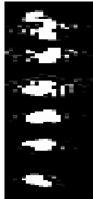
Figure 107: A typical scan appearance of samples perfused with manganese chloride at 6 concentrations. Scan time 40.8 s.
