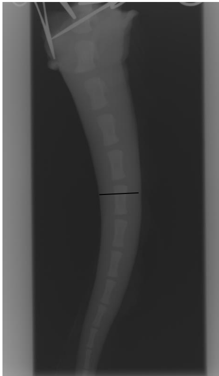
Figure 34: Pre-contrast sample; lateral, 60 kVp and 20 mA s. The lateral view enables a conclusion to be drawn if there is any difference in gray value depending on orientation.
