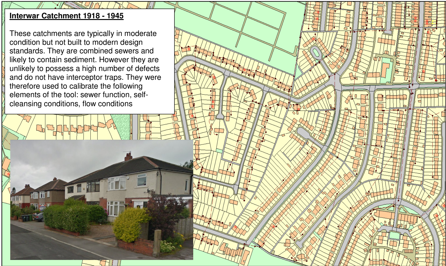
Figure 4-4 Overview of an Interwar 1918 – 1945 sewer system and parameters calibrated
