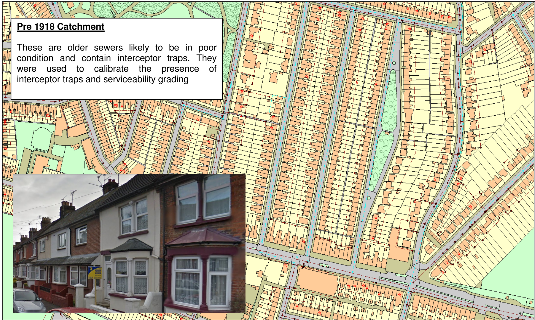
Figure 4-5 Overview of a pre 1918 sewer system and parameters calibrated
