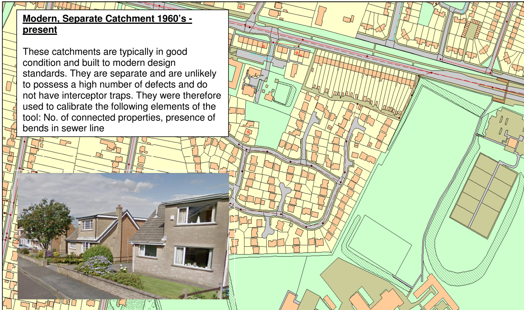
Figure 4-3 Overview of a modern separate foul sewer system and parameters calibrated
