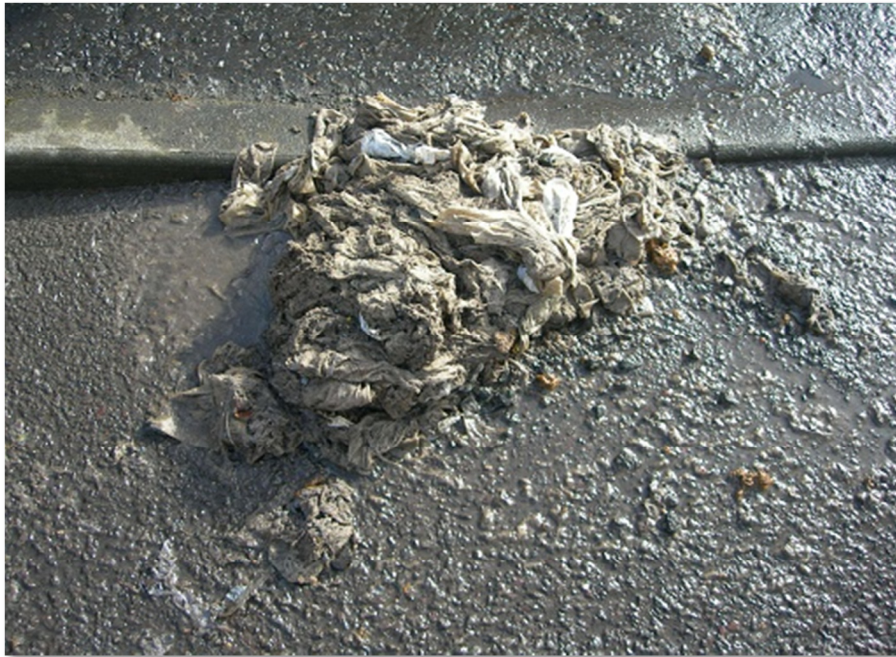
Figure 2-8 Coalesced sanitary wipes removed from a blocked sewer
