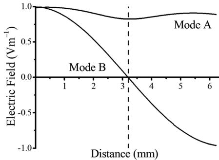
FIG. 3. Electric field profile for the two modes labeled as A and B in Fig. 2 plotted along a line in the  $z$  direction which passes through the center of a hole in the subwavelength mesh. Mode A was plotted at 7.42 GHz and mode B was plotted at 12.06 GHz.
