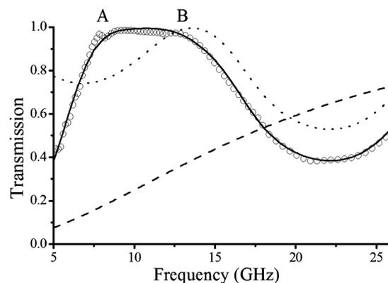
FIG. 2. Experimentally measured (circles), and numerically modeled (continuous line) normal incidence transmittance for the dielectric-clad subwavelength mesh shown in Fig. 1. The dashed line is the numerically modeled response of the unclad subwavelength mesh in free space and the dotted line is the modeled response of the sample without the metal mesh layer.
