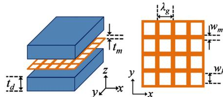
FIG. 1. (Color online) Left: exploded schematic of the experimental sample metallic mesh of thickness  $t_m=18\ \mu\text{m}$ , between two low loss dielectric layer  $t_d=3.17\ \text{mm}$  thick. Right: copper subwavelength mesh has a pitch  $\lambda_g=5.00\ \text{mm}$ , hole width  $w_h=4.85\ \text{mm}$  and therefore a metal “bar” width of  $w_m=0.15\ \text{mm}$ .
