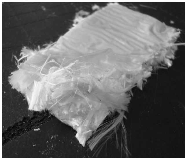
Figure 10: Poor fibre wet-out achieved in matured Rayon SMC
