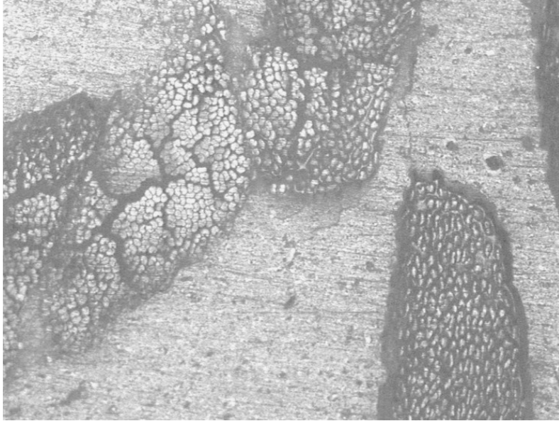
Figure 6: Poor separation of bundled 12k carbon fibre tow in CFSMC
