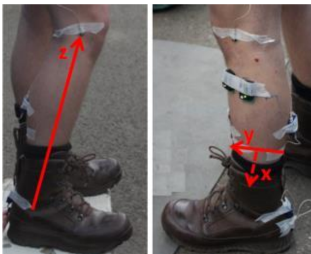
Figure 3.6: Axes of the shank segment (walking protocol)
