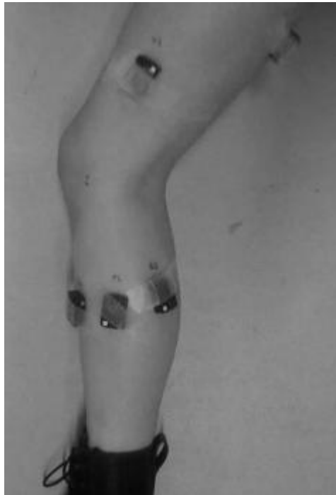
Figure 3.11: Positioning of EMG sensors on the left leg
