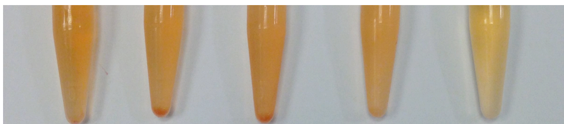
Figure 4.8: The selenium nanospheres formed in the presence of 0.5 \mu\text{g/ml} , 1 \mu\text{g/ml} , 5 \mu\text{g/ml} , 10 \mu\text{g/ml} and 50 \mu\text{g/ml} (from left to right) His-SefA-His.
