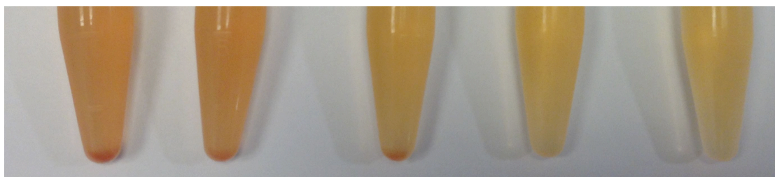
Figure 4.7: The selenium nanospheres formed in the presence of 0.5 \mu\text{g/ml} , 1 \mu\text{g/ml} , 5 \mu\text{g/ml} , 10 \mu\text{g/ml} and 50 \mu\text{g/ml} (from left to right) His-SefA.
