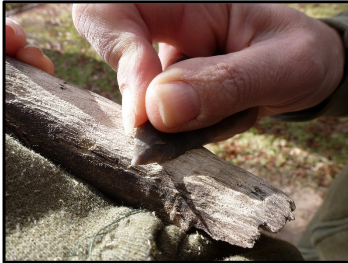
Figure 24. BB-02. Whittling the bark off a branch of dry willow for 60 minutes using experimental specimen BB-02.
