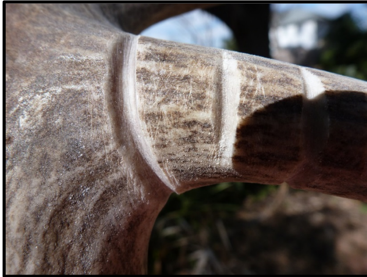
Figure 26. Grooves sawed into the tine of a white tail deer antler for 30 minutes using experimental specimen AS-04.
