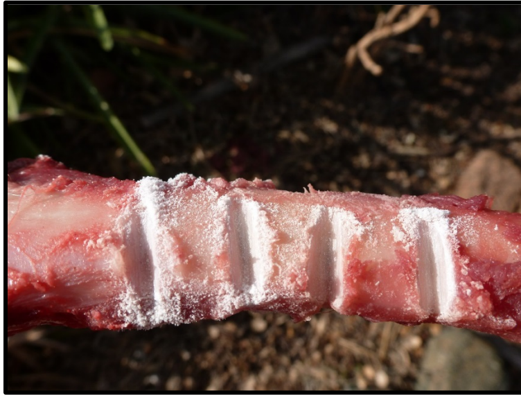
Figure 28. V-shaped grooves sawed into white tail deer bone for 30 minutes using experimental specimen AS-10.
