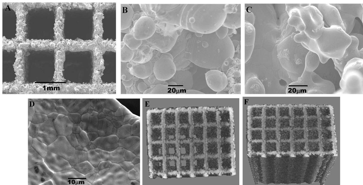
**Fig. 1** SEM images of the as-received 3D-printed Ni scaffold before (A, B) and after (C) annealing at 1370°C and the as-received random Ni foam (D); Micro-CT images of the 3D-printed Ni scaffold after annealing at 1370°C (E, F)
