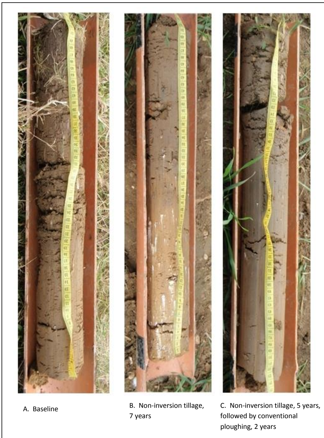
Figure 6.12: 50 cm cores taken from farm three. A: Baseline. B: Non-inversion tillage, 7 years. C: Non-inversion tillage, 5 years followed by conventional ploughing, 2 years.
