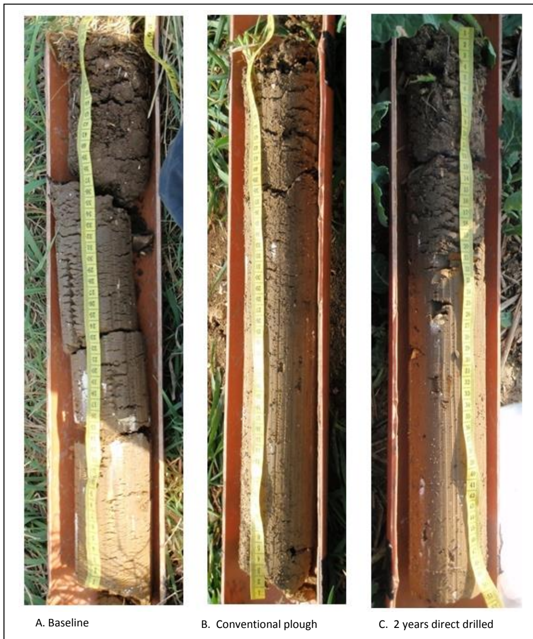
Figure 6 22: Three 50 cm cores taken from Farm six. A: Baseline, B: Conventional ploughing, C: 2 years direct drilling.
