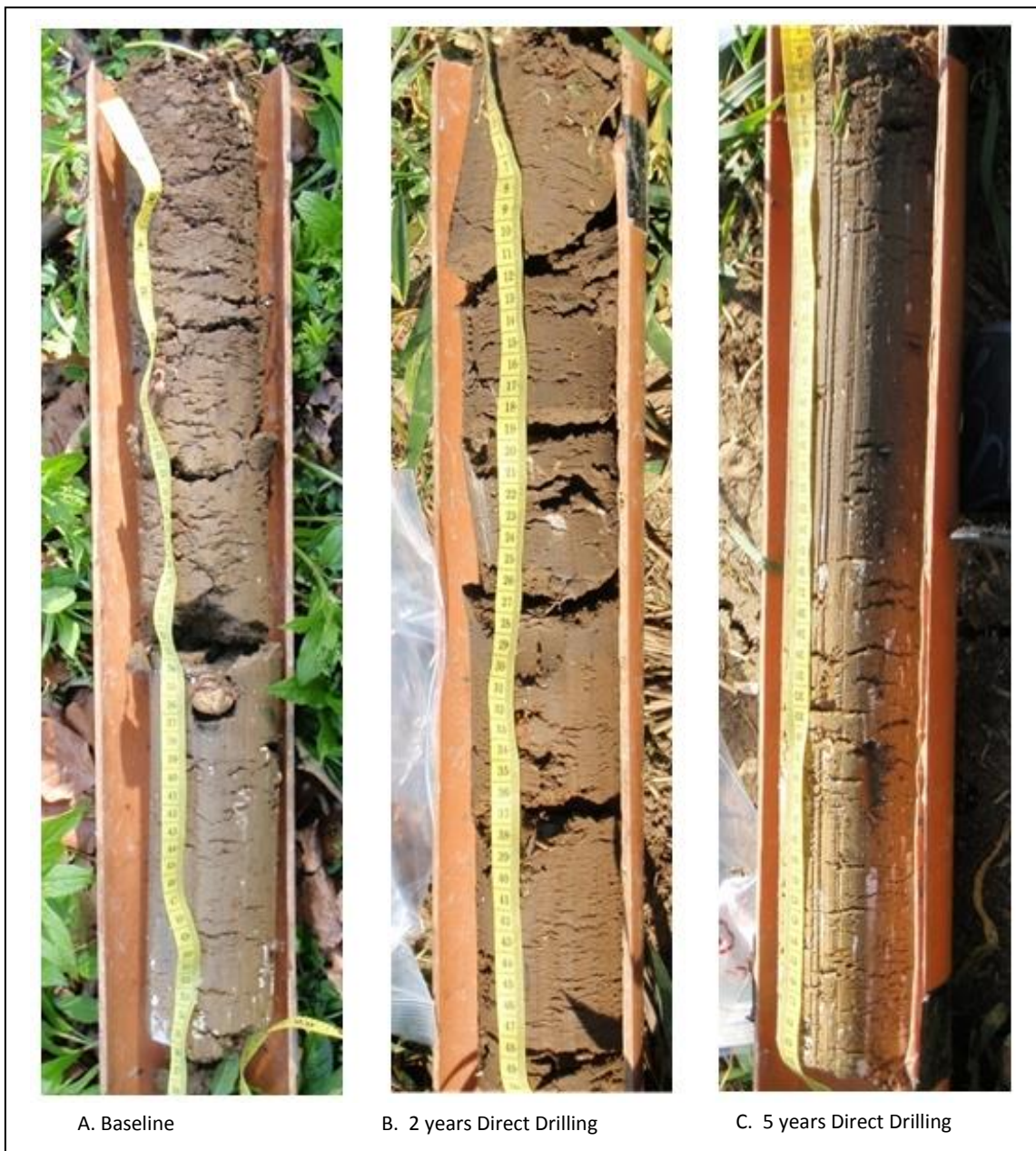
Figure 6.21: Three 50 cm cores taken from Farm five. A: Baseline, B: 2 years direct drilling, C: 5 years direct drilling.
