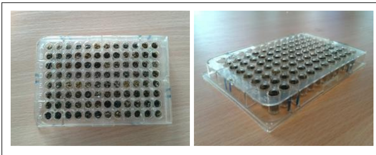
Figure 4.7: Soil samples placed into the 'wells' of plastic boxes ready for HCl fumigation.
