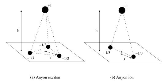
**Figure 3.** 'Classical' anyon exciton (a) and ion (b) in the planar geometry, where h is the separation between the electron and hole confinement planes and r is the distance between each anyon and the centre of negative charge. Note that charges are scaled by the electron charge e.
