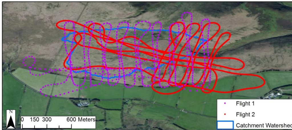
Figure 7.4 Flight paths for Unmanned Aerial Vehicle. Approximately 100 m altitude, 60 % along track overlap and 30 % across track overlap. The second flight path was at an oblique angle to the first, but still flying up-wind, to increase overlap.
