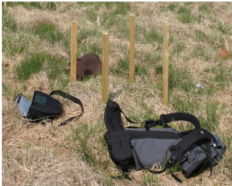
Figure 7.3 Typical placement of solid static objects with distinct colours around the vegetated plot to increase the probability of keypoint identification.
