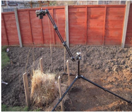
Figure 3.12 Tripod set up for downward facing images used to derive greenness excess index between 20/06/2012 and 25/10/2012.
