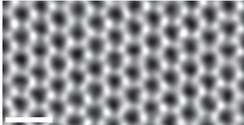
Figure 2.15: Atomic-resolution ADF-STEM image of a defect-free graphene crystal, showing the honeycomb lattice. The scale bar shows 5\text{\AA} [85]
