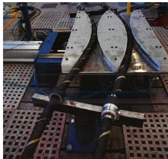
Figure 2: Bending against template test arrangement DMAc low cycles fatigue test
