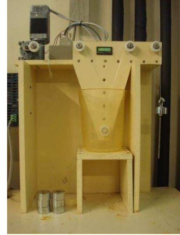
Fig. 2 Yarn-on-yarn abrasion test machine at IFREMER set up ready for testing (from [25])
