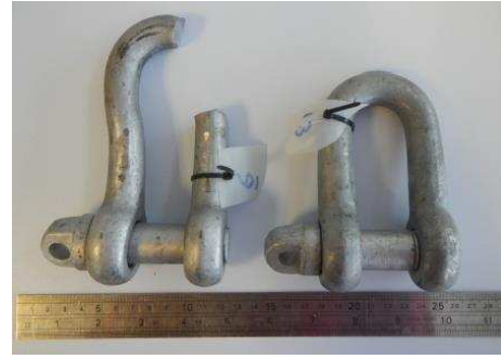
Fig. 5 Comparison of (left) failed shackle 6 and (right) undamaged shackle (from [26])
