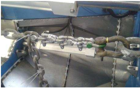
Fig. 4 Shackle setup in the DMaC test facility (from [31])
