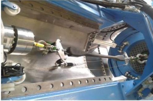
Figure 6: Technology for Innovation (TfI) mooring tether during performance and service simulation test at DMAc.
