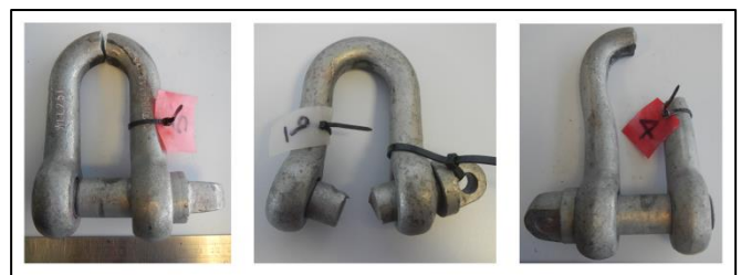
Figure 2: Examples of failed shackles
