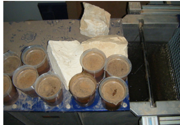
(b) Beakers with silty fine sediment suspension ready to be poured at the downstream end of the experimental channel, screen visible on the right.
