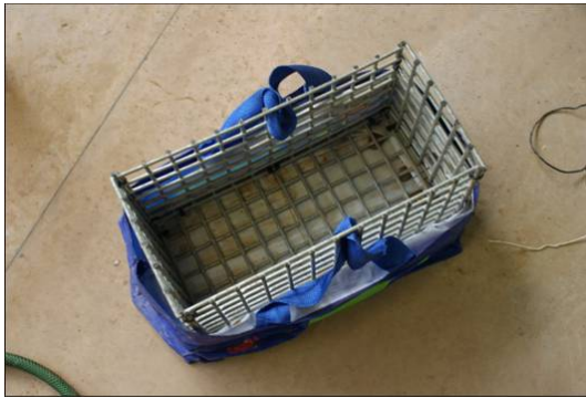
(a) Empty basket trap with folded sleeve before installing in the bed, wire with 2 mm diameter and 16 mm grid squares.
