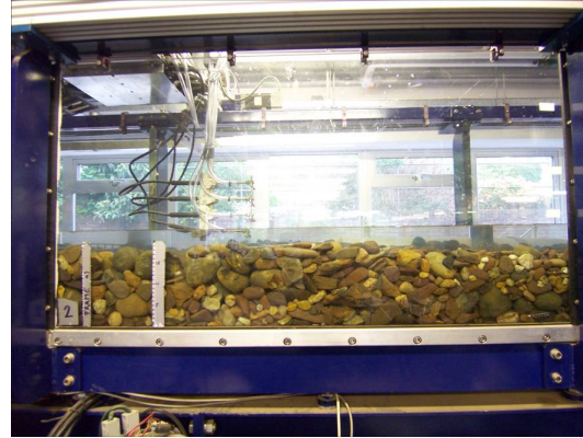
(b) Lateral view into experimental channel during fill up for S2Q30D48-1 with ADV heads mounted at 5, 10, 15 and 20 cm above the bed. Further the picture shows the sampling tubes used for concentration measurement at different heights which were attached to each head.
