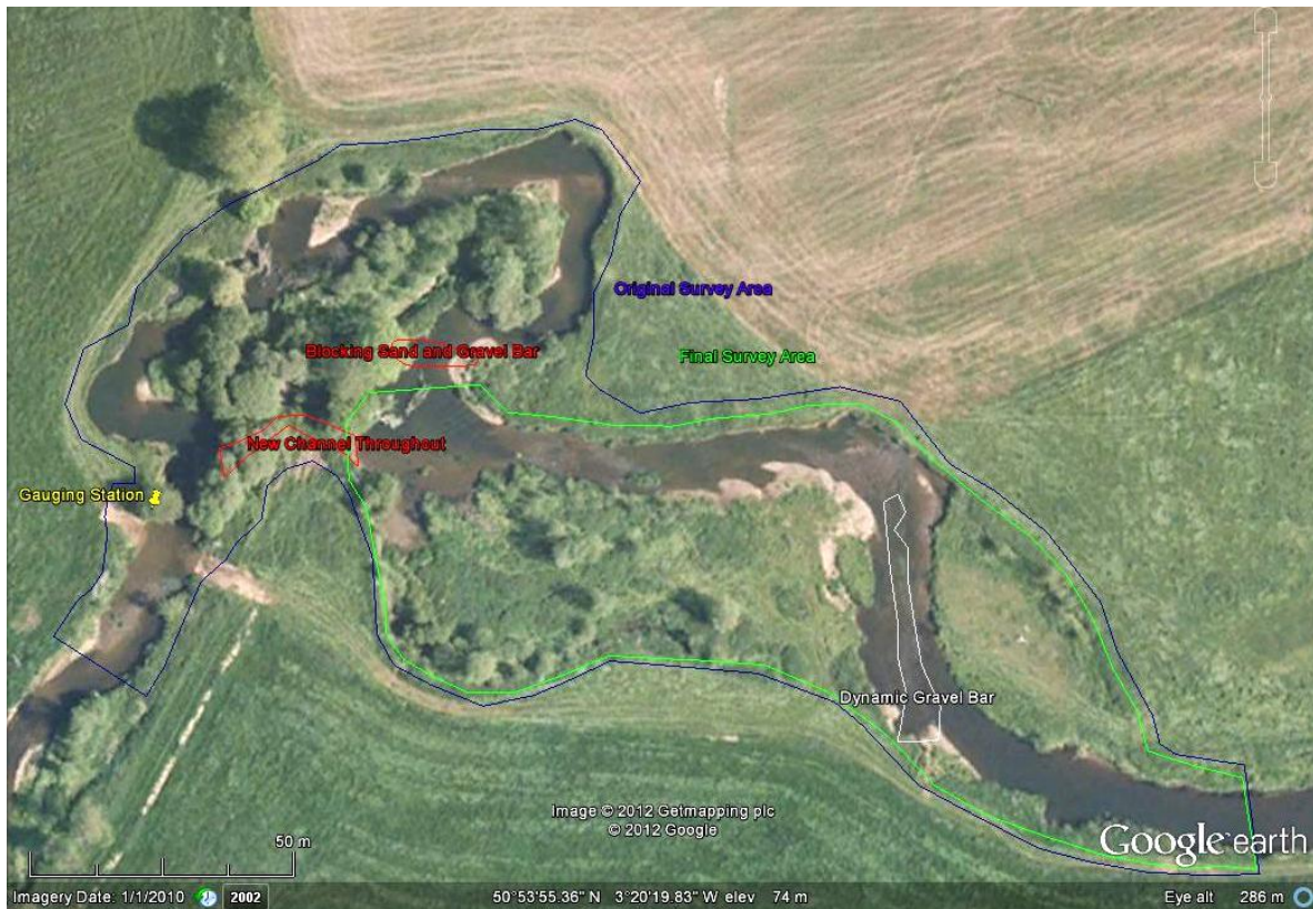
Figure 4.3: Satellite image of river channel and floodplain at Smithincott outlining the original study reach in blue, final study reach in green and a gravel bar which formed in December 2009 in white. The latter was not yet formed when satellite image was taken. The date (01/01/2010) watermarked on the Google image is not correct because, first, the gravel bar in the upper part of the reach is not visible, despite low water levels with exposed gravel and, second, trees are foliated. It seems plausible that the picture was taken in summer 2009. Additionally, new features appeared between 2010 and 2011 in red, these features being a gravel bar blocking inflow in the lower meander bow and a new cut through connecting the upper part of the reach directly to its outlet.
