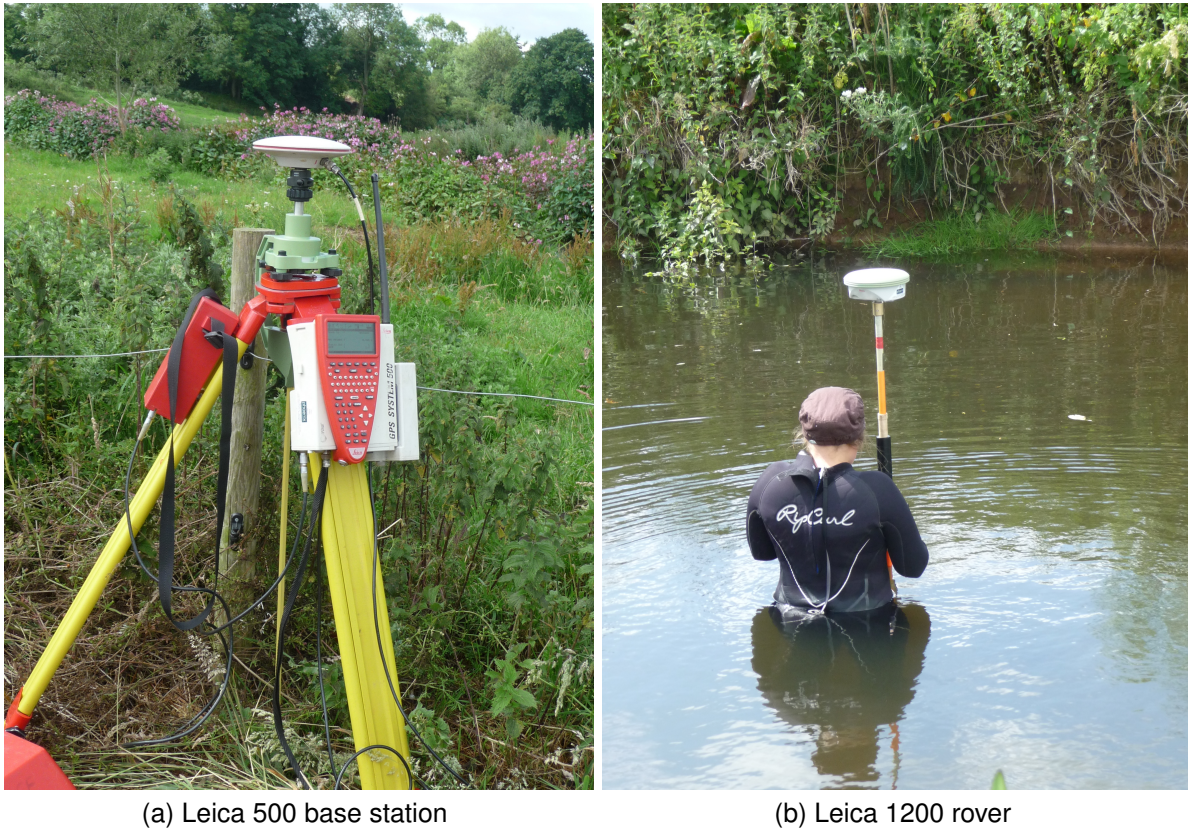
Figure 4.9: Differential GPS used for the elevation survey with a base station for exact reference and mobile rover for detailed mapping of river bed, bank and floodplain
