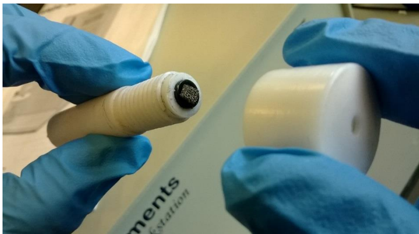
Fig 3.7 Mounting GF on a working electrode by using a Teflon holder.
