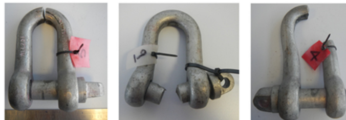
Figure 2. Examples of failed shackles.
