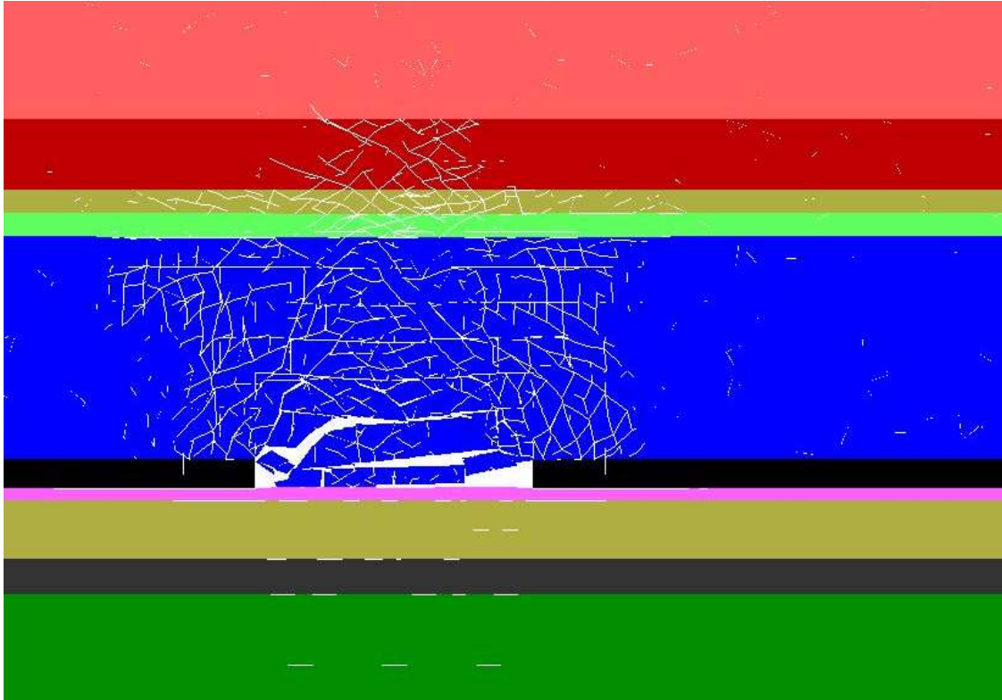
Fig. 18 Simulated fracture pattern in model with weak immediate roof. The roof ruptures when the face advances 24 m.
