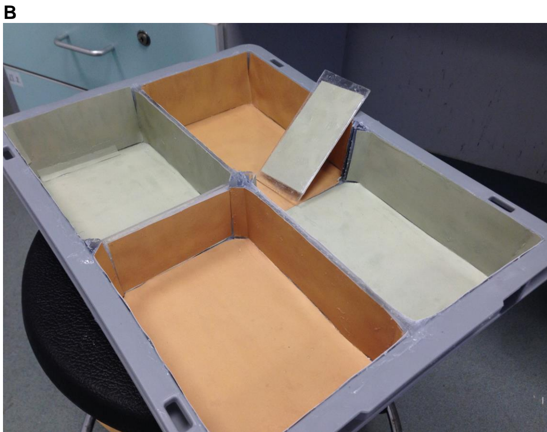
Figure 2.1: Experimental tray used for experiment 1. (A) Diagram showing the experimental backgrounds and the design of the tray used in experiment 1, and (B) final tray with one of the sliding dividers removed. Note that colours of the backgrounds may not be a true representations of the actual colours used in the experiment. Photo credit: Sam Smithers
