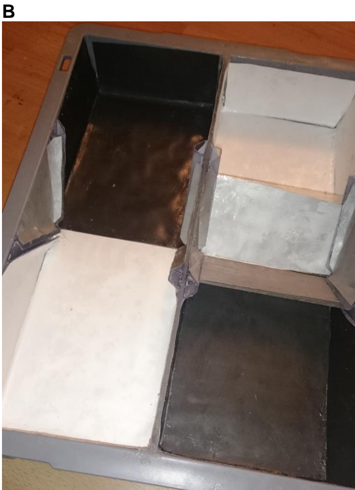
Figure 2.4: Experimental tray used for choice tests in experiment 4. (A) Diagram showing the experimental backgrounds (same as the black and white used in experiment 2) and the design of the tray used for experiment 4, and (B) final tray with the starting dividers on one side removed. Note that colours of the backgrounds may not be true representations of the actual colours used in the experiment. Photo credit: Sam Smithers
