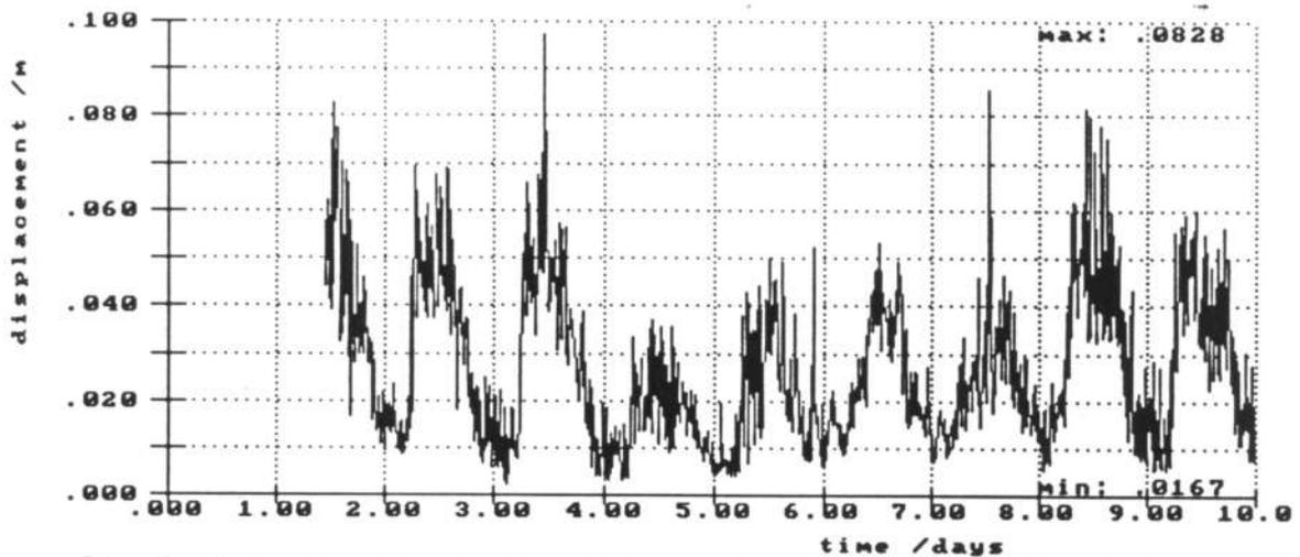
Standard deviation of vertical displacement of deck at centre span
