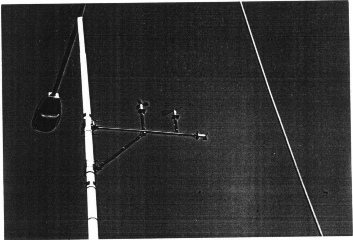
Fig. 5a Installation of cup anemometer and vanes on lamp post
