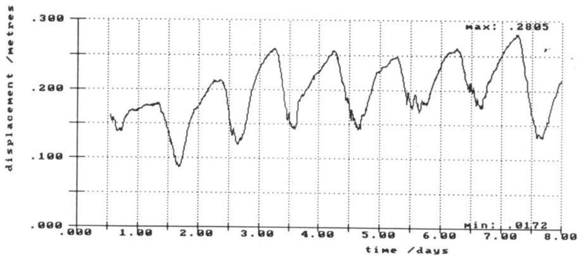
c) Longitudinal displacement away from Hesse tower
