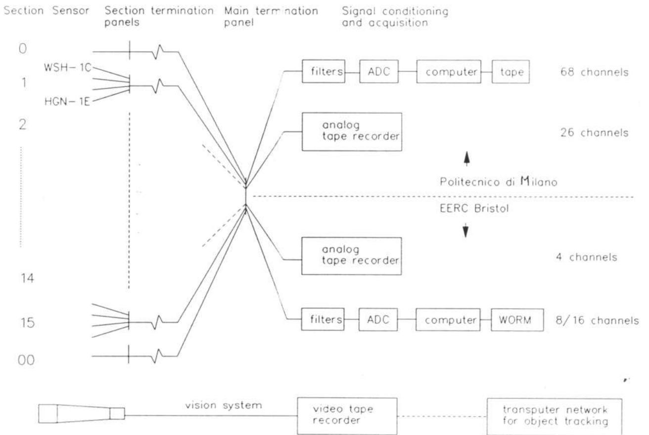
Fig. 7 Overview of data acquisition system
