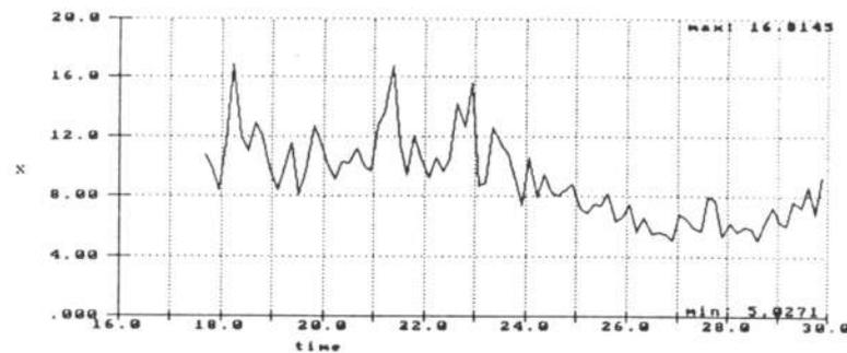
e) Turbulent intensity  $I = \sigma(V) / \mu(V)$
