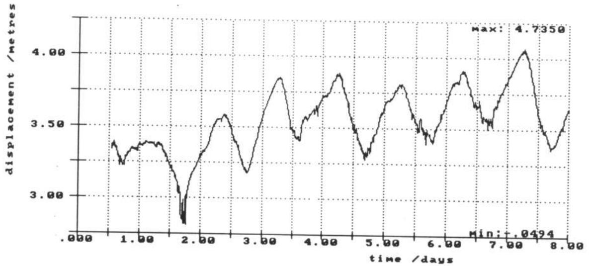
b) Vertical displacement at midspan
