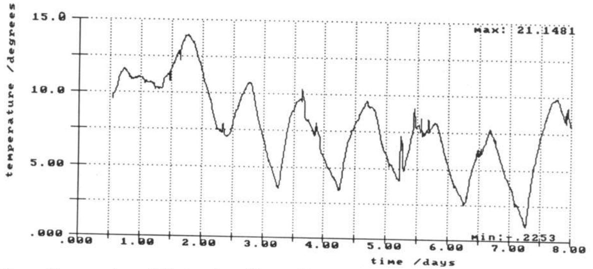
a) Temperature of East main cable at mid-span
