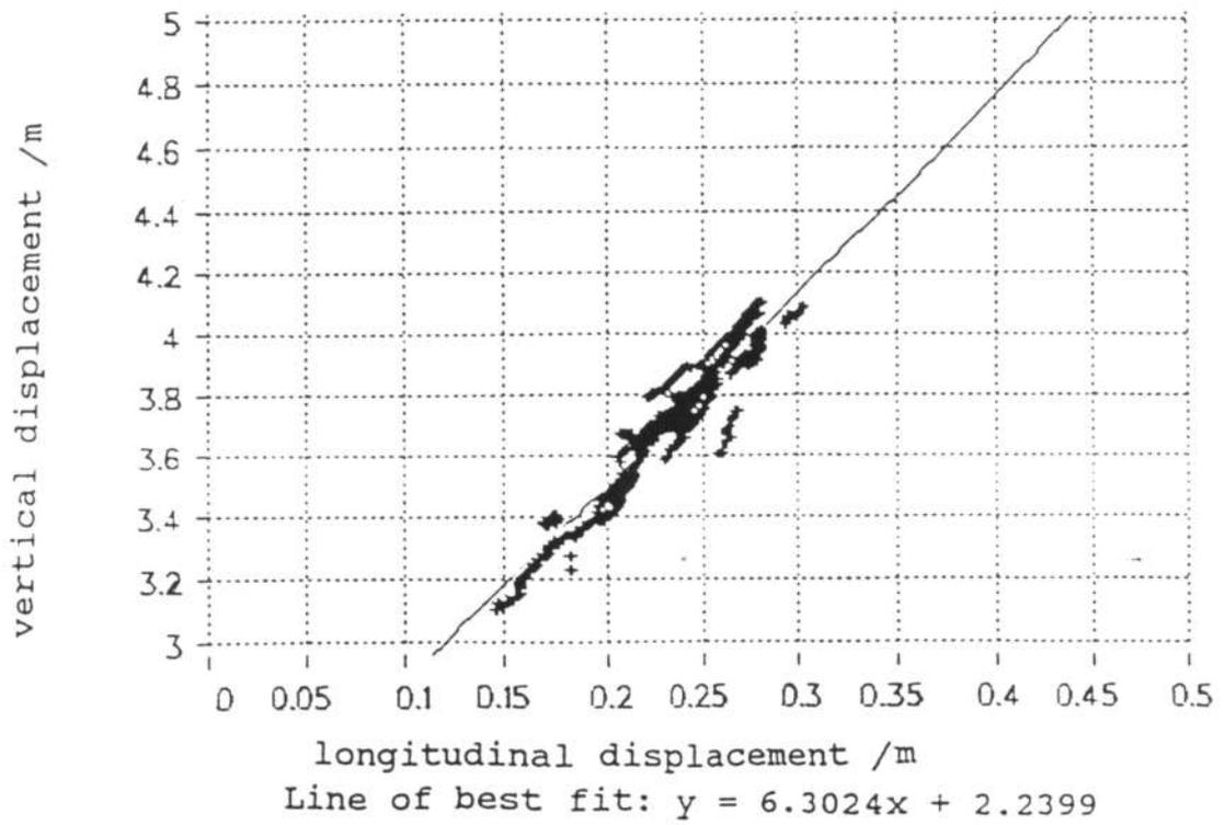
Fig. 12 Longitudinal displacement (away from tower) vs. vertical displacement
