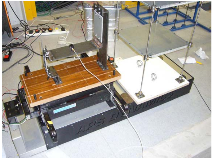
Figure 4 Folded pendulum performance test
