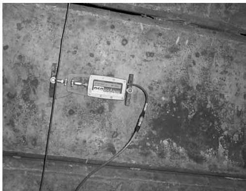
(b) Demountable strain gauge
