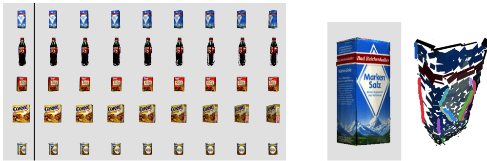
Fig. 17 Left: Example prototype views (leftmost column) and test images, all shown only by left view of the stereo images, for a subset of the tested KIT objects. Right: left view of a virtual stereo input image of the KIT object “BlueSaltCube” (leftmost) and the extracted contours and surfings from the virtual stereo image (rightmost).
