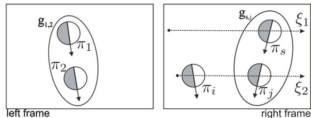
**Figure 8. The BSCE criterion.** Let  $\pi_1$  be a primitive in the left frame forming a group with a second primitive  $\pi_2$ .  $\pi_1$  has a stereo correspondence  $\pi_s$  that lie on the epipolar line  $\xi_1$  in the right image. Both  $\pi_i$  and  $\pi_j$  in the right image lie on the epipolar line  $\xi_2$  of  $\pi_2$ ; hence these two primitives are both putative correspondences of  $\pi_2$ . doi:10.1371/journal.pone.0010663.g008
