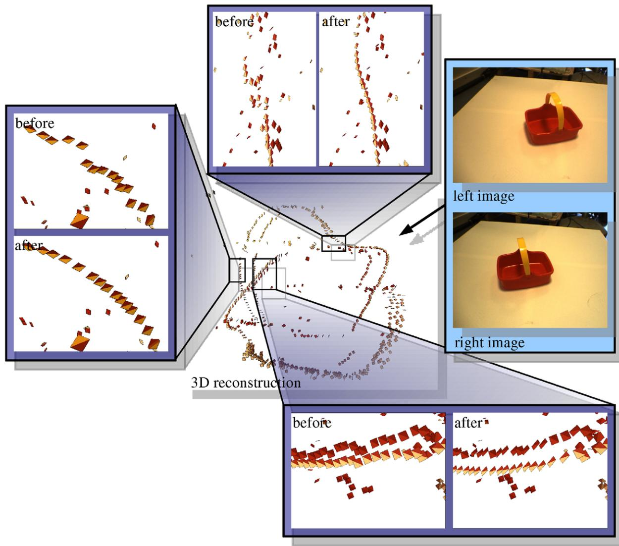
**Figure 19. Illustration of the effect of the correction of 3D primitives using interpolation.** The figure shows the reconstructed primitives before and after 10 rounds of correction, for details of an object.
