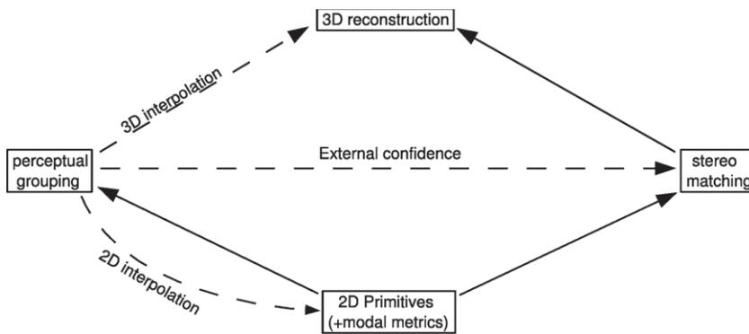
**Figure 1. Summary of the scheme presented in this paper.** In this figure, solid arrows mean direct dependencies and dashed lines corrective feedback.
