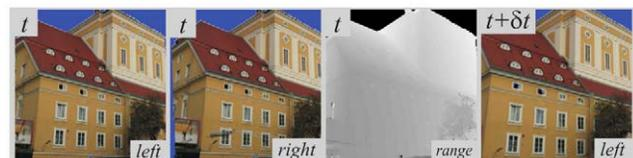
**Figure 9. Illustration of how a sequence is generated from colour range images.** The images show the first  $t=1$  left and right images, the left disparity image, and the last left image ( $t + \delta t = 10$ ). doi:10.1371/journal.pone.0010663.g009
