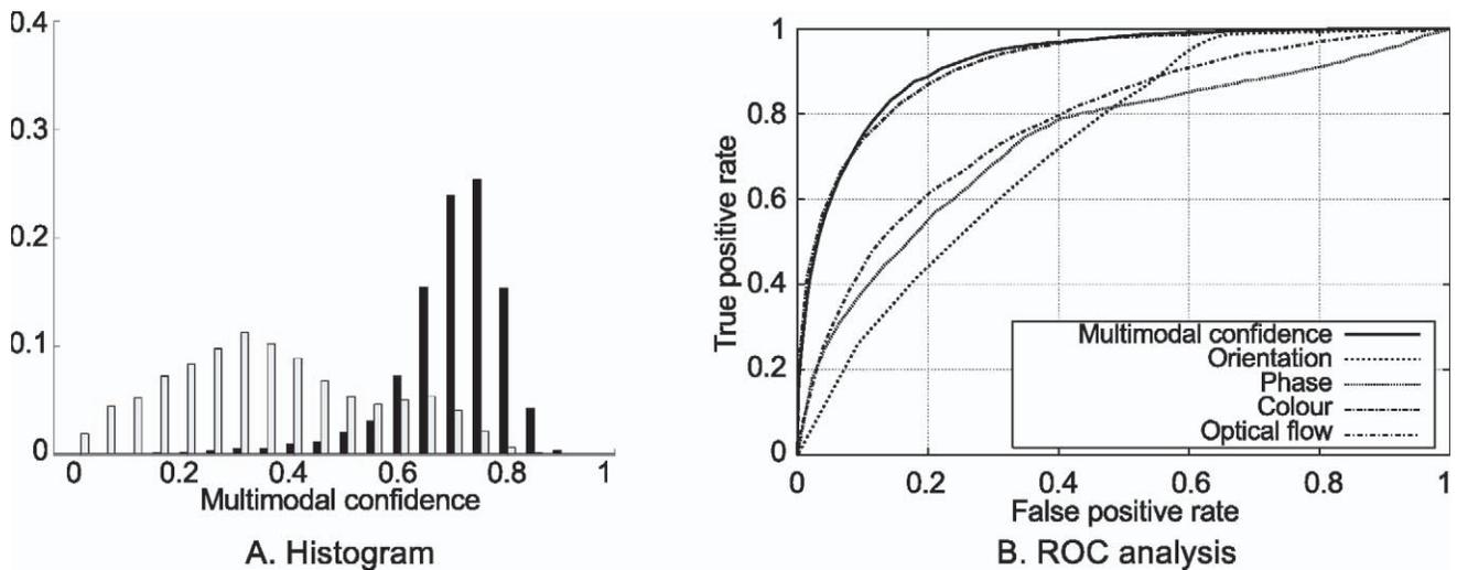
**Figure 12. Evaluation of the multi-modal stereo.** **A** Histogram of the multi-modal similarities between correct (black bars) and false (white bars) potential correspondences. **B** ROC curves for the different modalities. These results have been collected over 10 frames of the sequences Figure 10 **A**, **B** and **C**.
