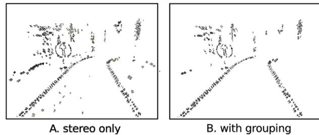
**Figure 14. Qualitative example of the effect of the external confidence threshold.** **A** primitives reconstructed from the sequence in Figure 10D, without threshold on external confidence ( $\tau_m = 0.8$ ,  $\tau_e = -1.0$ ). **B** primitives reconstructed from the same sequence with a threshold on external confidence ( $\tau_m = 0.8$ ,  $\tau_e = 0.1$ ). doi:10.1371/journal.pone.0010663.g014
