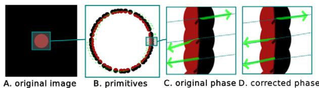
**Figure 17. Illustration of the effect of phase correction in 2D.** A the original image; B the extracted primitives; C detail of the primitives, the green arrows show the extracted phase, the dotted lines show the mean phase over the whole circle; D detail of the primitives after correction: the central primitive's phase is now closer to the dotted line. doi:10.1371/journal.pone.0010663.g017
