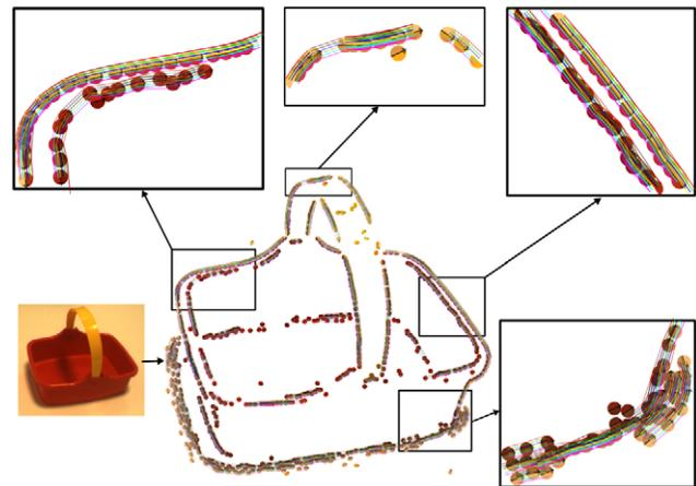
**Figure 6. Illustration of the affinities between 2D primitives.** In this figure, the 2D primitives are linked by coloured lines, where a brighter colour stands for a stronger affinity. Red stands for collinearity, green for phase, blue for colour and yellow for optical flow affinity. doi:10.1371/journal.pone.0010663.g006
