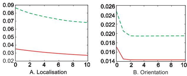
**Figure 18. Correction of 3D primitives.** Error of the **A** localisation and **B** orientation of the reconstructed 3D primitives after several iterations of the correction process. Solid lines shows the errors for the triangle scenario and dashed line for the circle scenario. The horizontal axis shows the number of iterations of the correction process and the vertical axis shows the error in **A** units (in the 3D space, arbitrary in an artificial scenario) and **B** radians.
