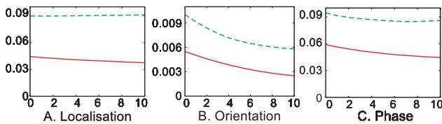
**Figure 16. Correction of the 2D primitives using interpolation.** Accuracy of the 2D primitives' localisation (A), orientation (B) and phase (C) after several iterations of the correction process, for the triangle (full line) and circle (dashed line) scenarios. The horizontal axis shows the number of iterations of the correction process and the vertical axis shows the error for A in pixels, and for B and C in radians. doi:10.1371/journal.pone.0010663.g016
