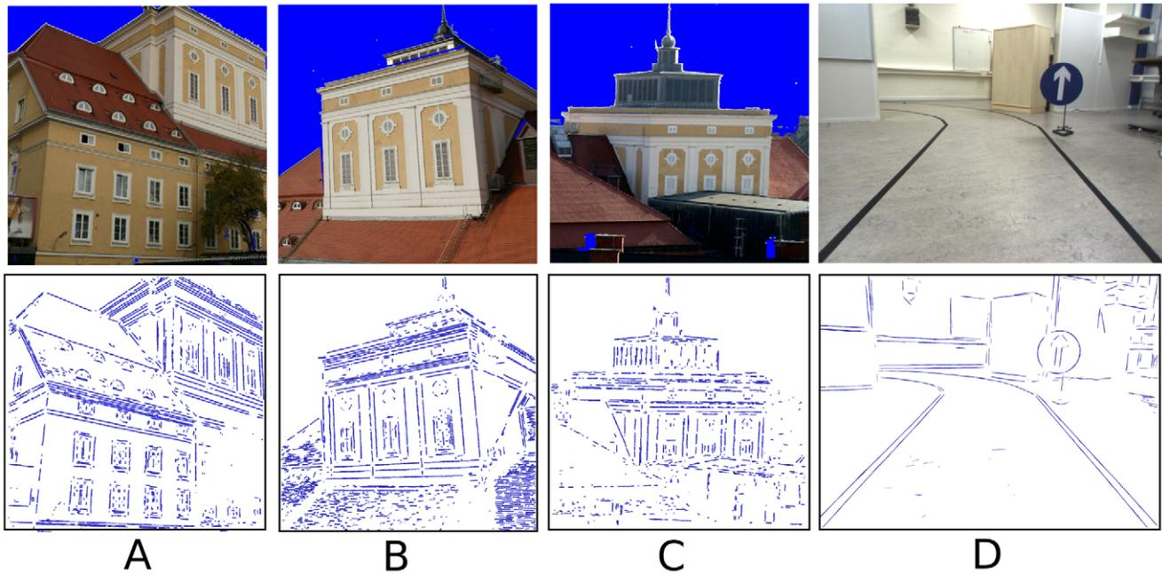
**Figure 10. The four sequences on which we tested our approach.** The top row shows one image from each sequence, and the bottom row shows the groups created.
