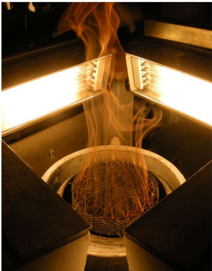
Flaming ignition of Pinus pinaster needles
