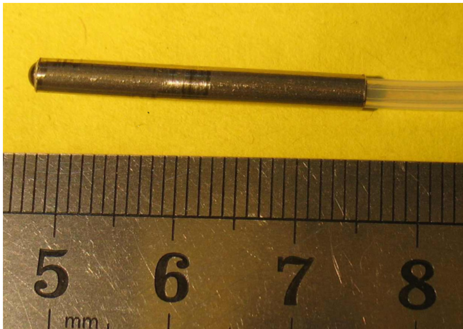
Figure 2-5 A) Schematic diagram of Raman probe. B) Packaged probe.
