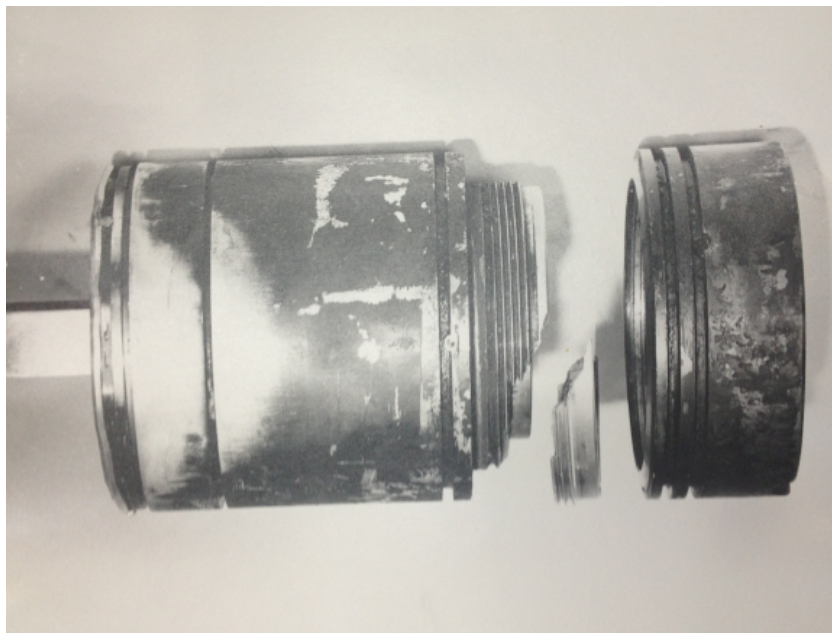
Fig 8 Photograph of failed piston recovered from Deltic generator, Perim Island (National Archives/FO/953/2230)
