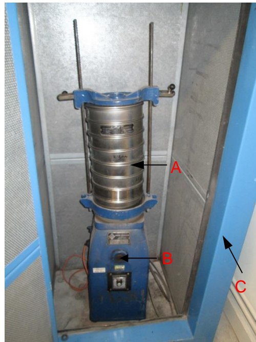
Figure 3.6 Pascal Engineering machine sieve shaker at CSM (CSM, 2015), A) Stacked sieves, B) timer C). Acoustic enclosure it's about 640 mm tall and 200 m wide.
