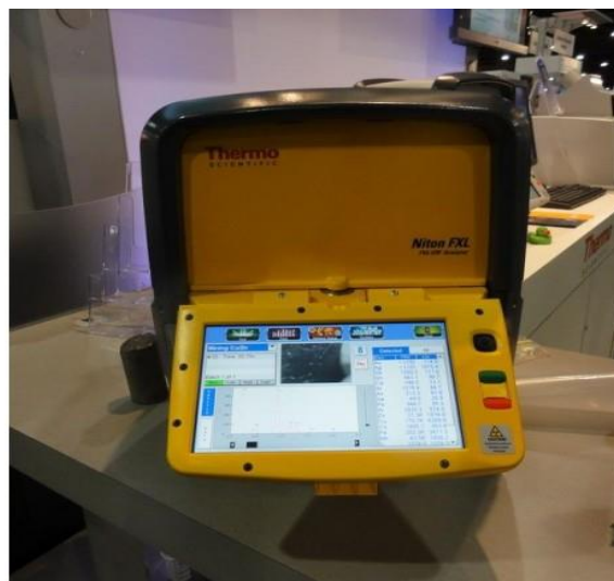
Figure 3.8 PXRF Niton FXL 950 FM-XRF analyser at CSM (CSM Laboratory, 2013)
