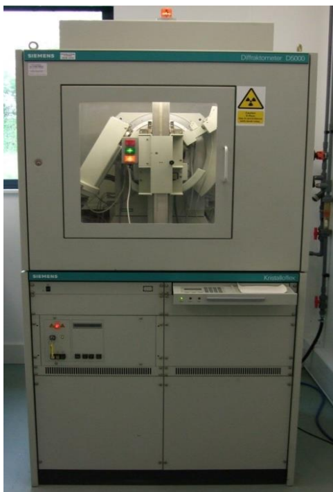
Figure 3.7 XRD Siemens D5000 at CSM (CSM Laboratory, 2015).
