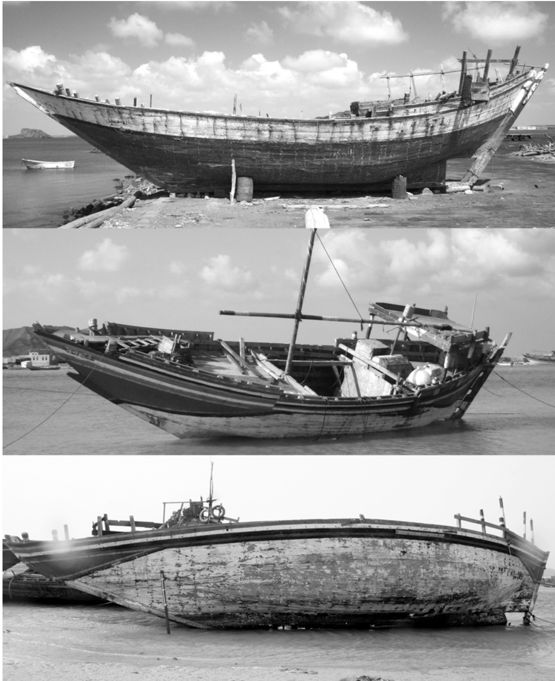
Figure 5: Three types of double-ended sanbūq found in Yemen – the ‘obrī (top) in Aden, and zārūq (centre), and zaīmah (below), in al-Ghureira (MARES/J.P. Cooper, C. Zazzaro).
