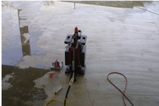
Fig. 5: The left photo shows a shaker and accelerometer that was used in phase 1 and the right plot shows the bare structure of phase 1
