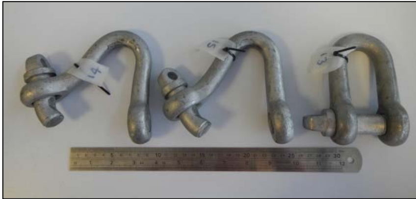
Figure 5: Shackles from Break Test 1, Break Test 2 and an undamaged shackle for reference
