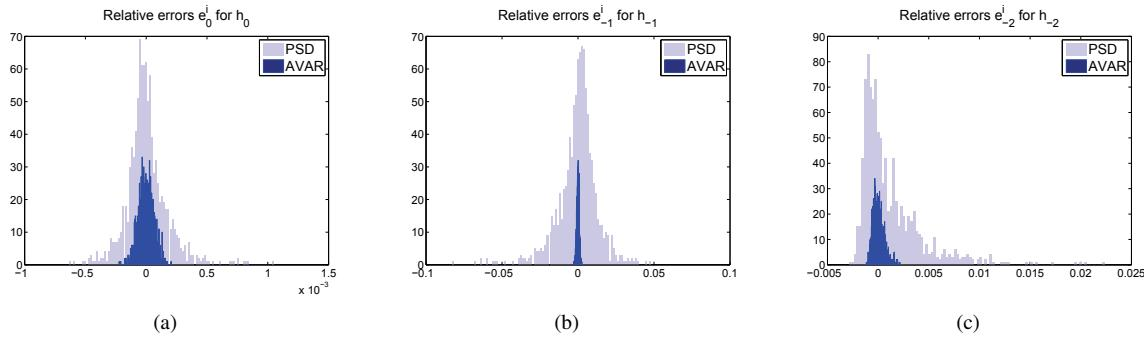
Fig. 2. Distribution of the relative estimation errors for  $h_0$  (a),  $h_{-1}$  (b), and  $h_{-2}$  (c) coefficients using AVAR. The results obtained from direct estimation using periodogram are also presented which are denoted as PSD in the above figures.
