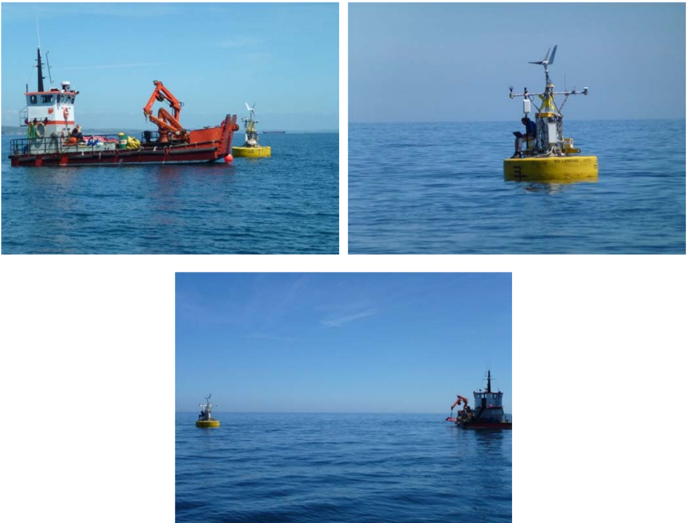
Figure 10: Deployment of the SWMTF
