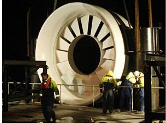
Open-Centre Turbine, developed by Open Hydro. Source: http://www.openhydro.com/company.html
