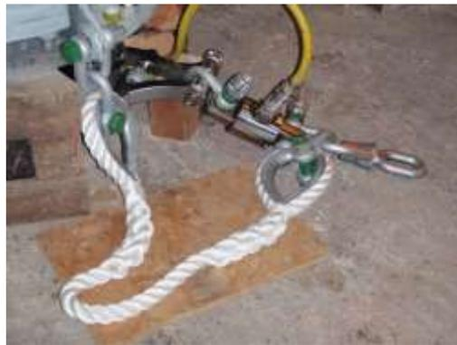
**Figure 5:** Example safety rope used on one mooring connection point of the SWMTF
