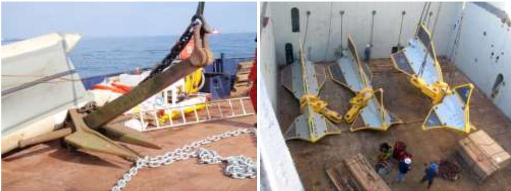
**Figure 4:** (left) 1.1 Tonne Danforth fluke anchor prior to deployment with the South West Mooring Test Facility<sup>4</sup>, (right) vertically loaded Delmar OMNI-Max anchor (source: Delmar Systems Inc.)
