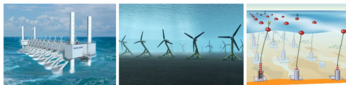
Figure 1. Artist's impressions of MRE arrays: (left) Wave Star wave energy converter (Marquis et al. 2010), (middle) ScottishPower Renewables Sound of Islay 10MW tidal turbine array (Carrell 2011), (right) Uppsala University wave power plant (Astrand 2013)
