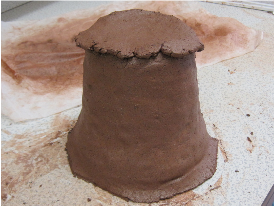
Figure v: Mounting of 75 % soapstone vessel bottom. The clay body was rested on the wall slab before subsequently being cut to shape after the bottom slab was fixed.
