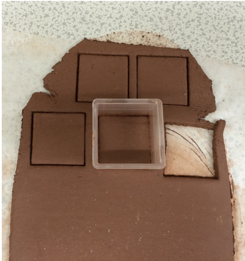
Figure viii: Manufacture of test-tiles. The paste was rolled to 5 mm thickness using rolling pin guides, and pressed out with a 45x45x50 mm plastic cookie cutter.
