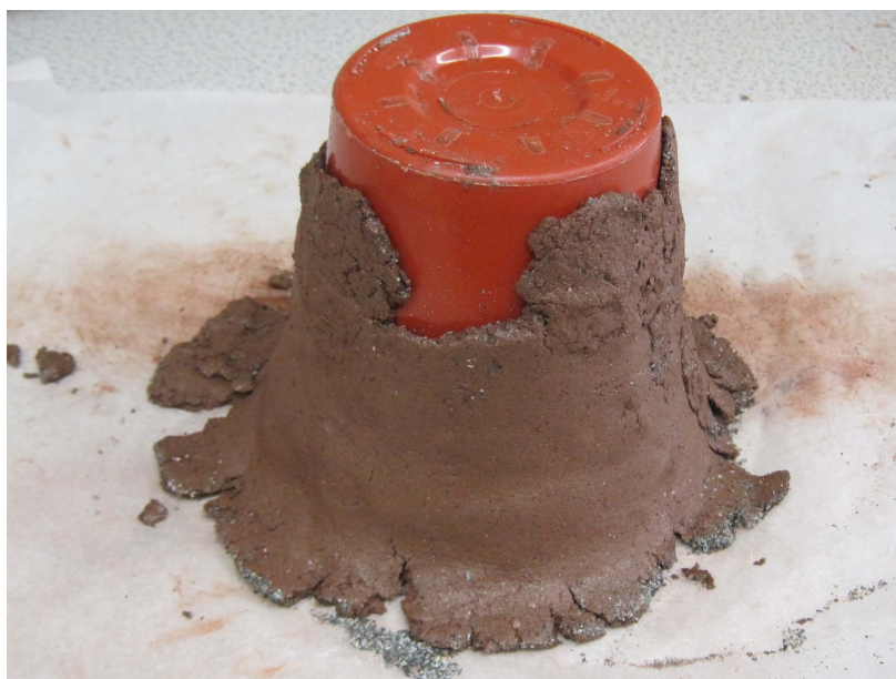
Figure 12: Moulding the test vessels. Note that the 75 % paste is being used to support itself on the table to prevent rupture, and patches are mended with additional, smaller slabs.
