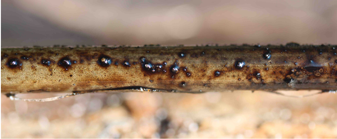
Figure 45: Tar bubbles on the thermocouple tube, experiment 3-3a (5 cm cover T).
