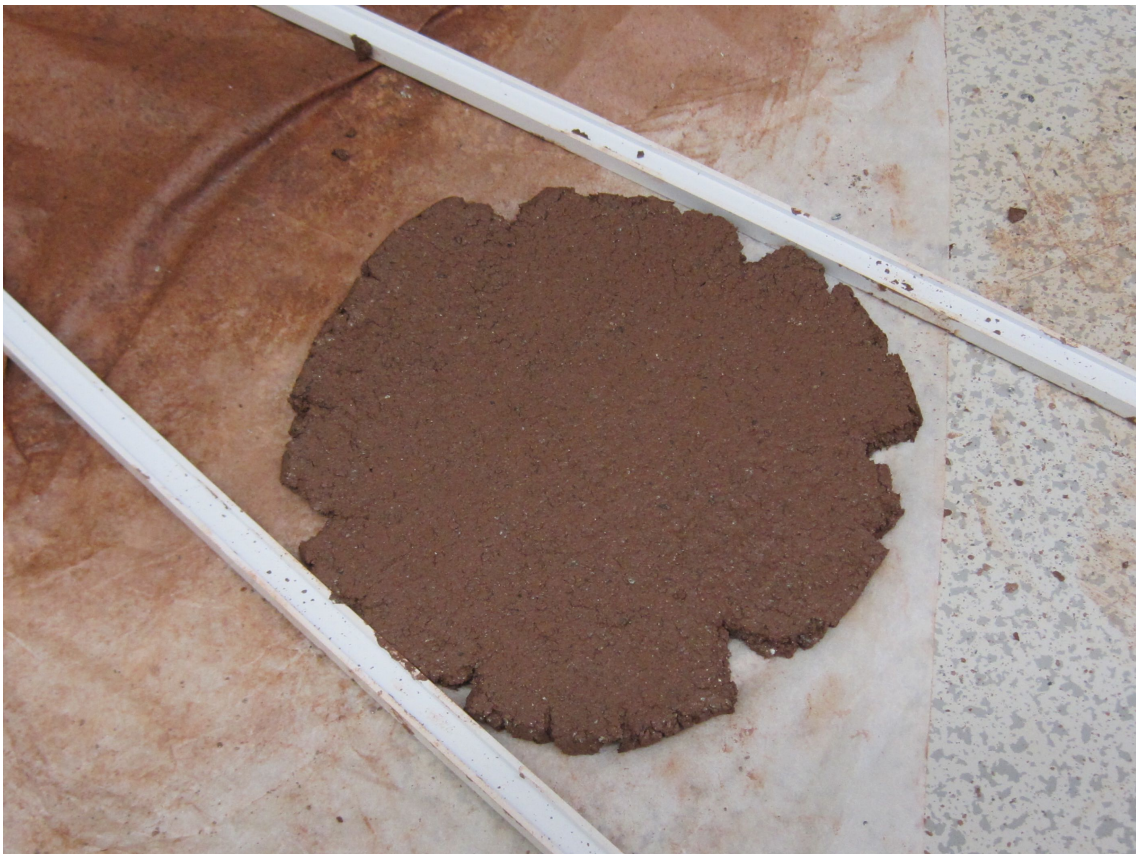
Figure iv: Preparation of 75 % soapstone slab for vessel bottom. The rolling pin guides (5 mm) were used consistently throughout experiment for all slabs used to manufacture the experimental vessels.
