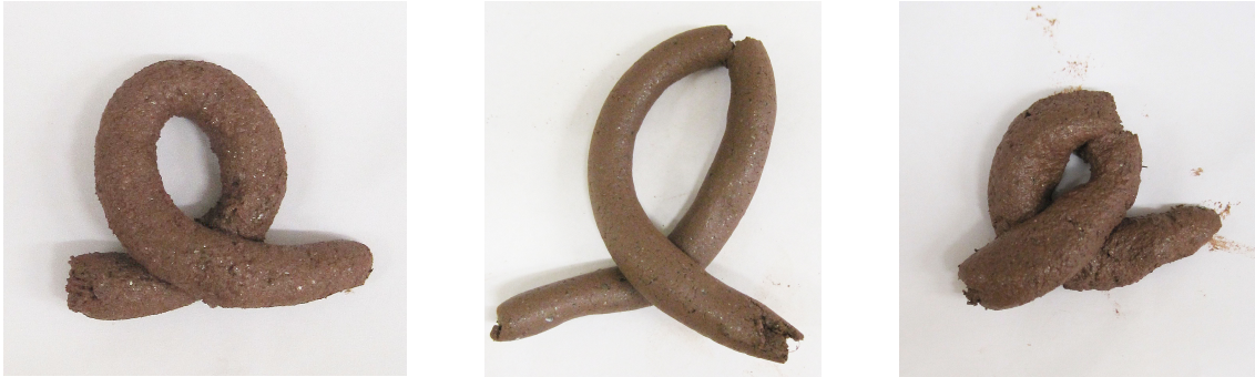
Figure i: Coil test of the tree clay pastes used in the experiment. This test shows illustrates unsuitability of the paste to be used for coiling due to lack of adhesion in archaeological soapstone blends. From left: 25 % soapstone, 50 % soapstone, 75 % soapstone. Clay: Etrurian marl, Red Earthenware Powdered Clay 1135/2, Bath Potter's Supplies, UK. Soapstone: Vargavågen, Os, Hordaland, Norway. This mix was used for all experiments apart from pilot experiment, where the latter was used with a commercially bought, wet terracotta clay. Photos: Author
