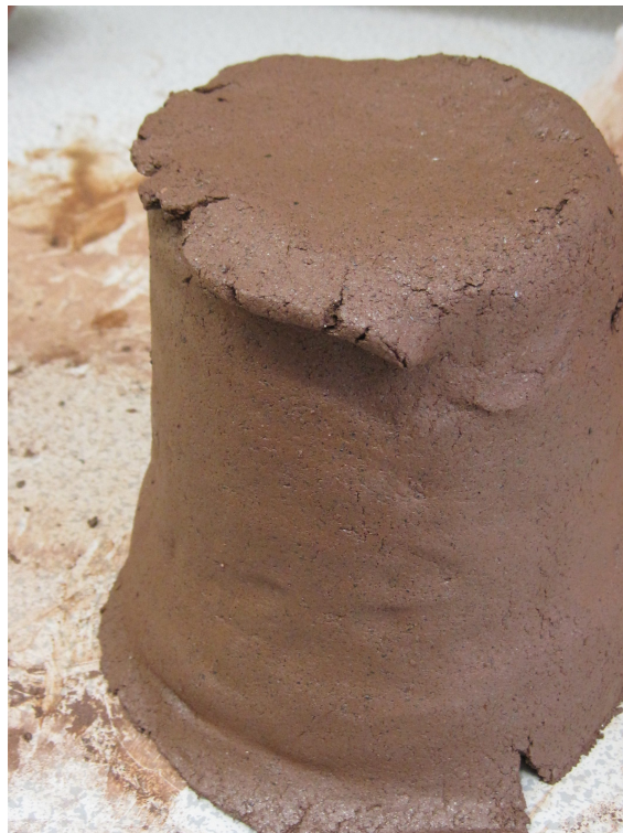
Figure vi: Mounting of 75 % soapstone bottom slab. Note the cracking that results from lack of adhesion in the paste. Due to this, the slabs were consequently laborious to adhere, and caution had to be undertaken in the process.
