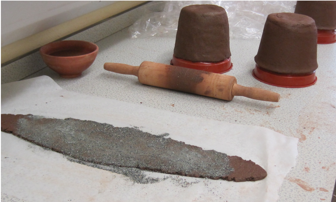
Figure iii: Preparation of 75 % soapstone slab for vessel wall. Note the covering of powdered soapstone to prevent sticking. Upon firing this becomes a loose powder that can be brushed off the interior wall if necessary.
