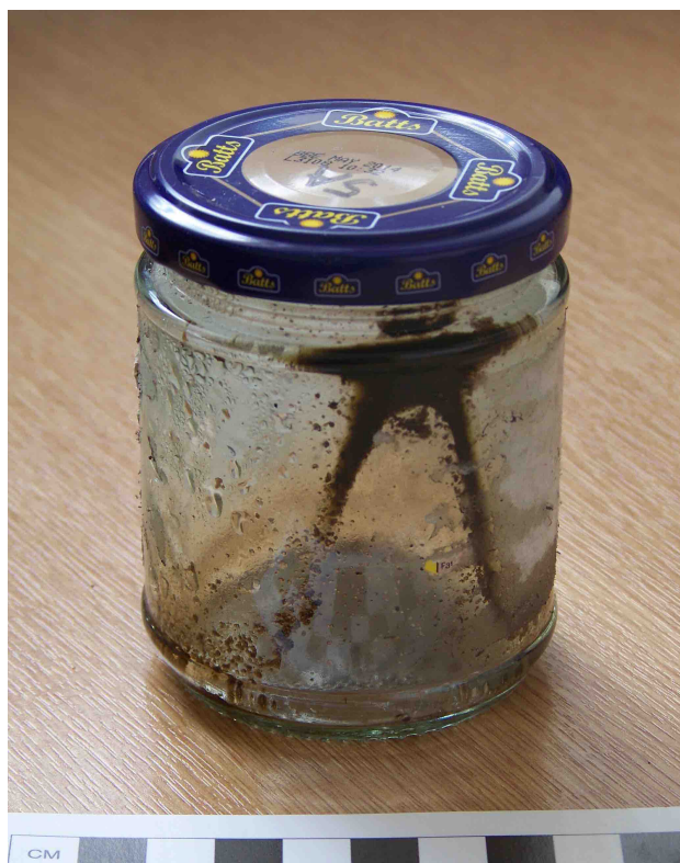
Figure 49: Tar from structure 3-5a (5 cm cover thickness). The star-shaped wall pattern is the outlet point of the collection tube and resulted from the jar's horizontal position in the ground. This photo was taken two weeks after the experiments, and some of the viscous pitch still clings to the vessel wall.
