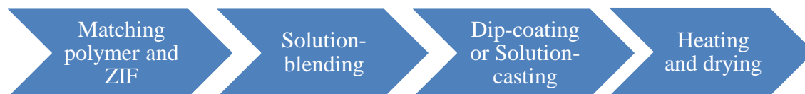
Figure 2.9 Basic procedures for the preparation of mixed matrix membranes.
