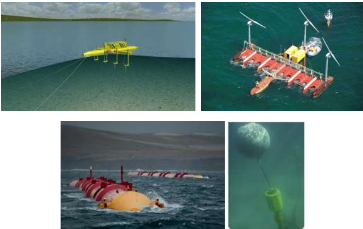
Figure 7: Example WEC devices ( top left ) Bluewater BlueTEC floating platform and ( top right ) Poseidon Floating Power platform. ( bottom left ) Pelamis Wave Power P2 wave energy converter and ( bottom right ) Carnegie Wave Energy CETO wave energy converter
